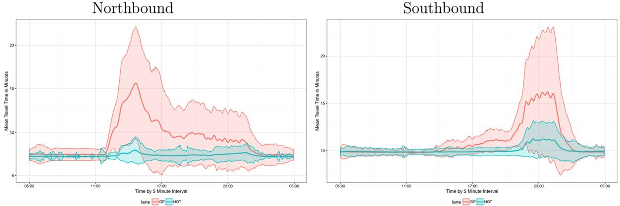
*Notes:* The thick line the mean travel time and the shaded region bounded by the thin lines represents one standard deviation in travel time. The colors distinguish between the GP and HOT lanes. Free flow travel time is approximately 10 minutes in either direction. The graphs consist of 1,566 days of 5-minute traffic data.
