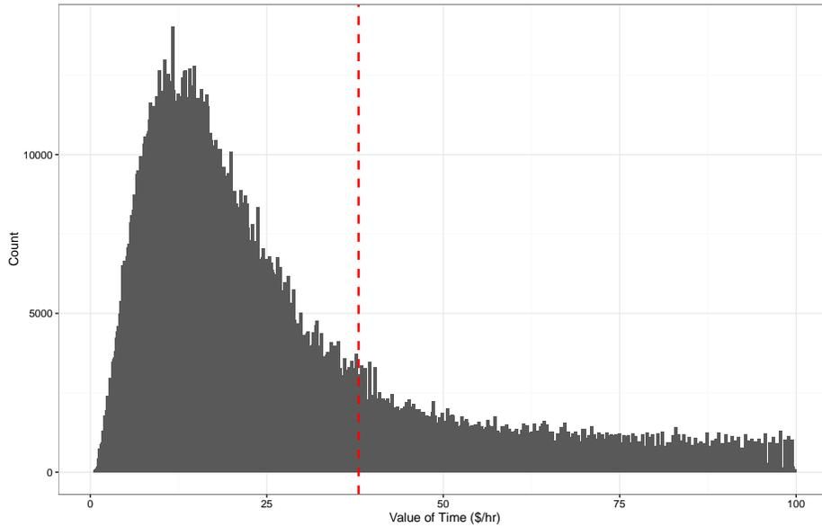
*Notes:* Simple VOT is based on toll and loop detector data. The red dashed line is the average. The figure does not show negative values or values above \$100/hr to assist in the viability.
