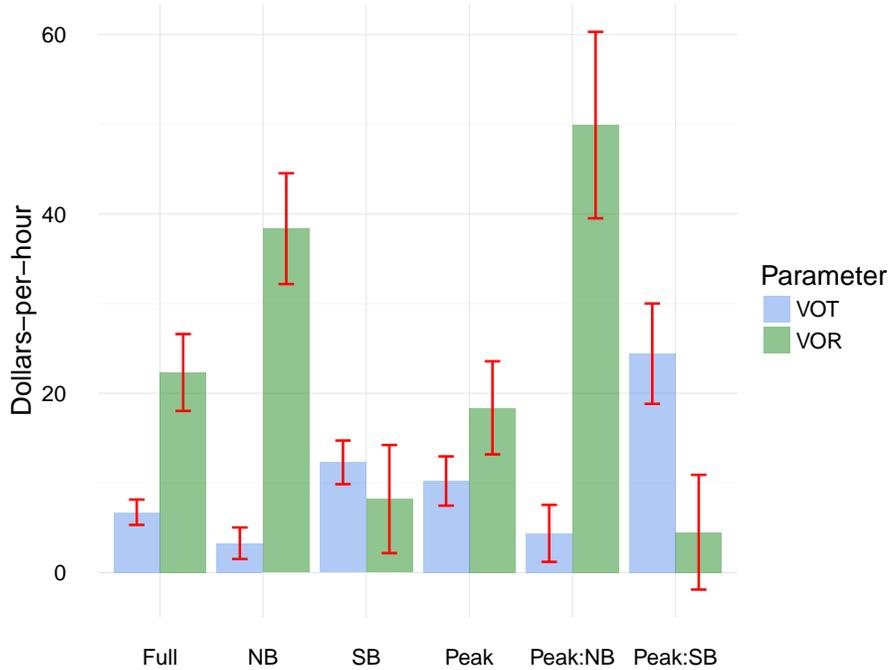
*Notes:* The thick bars are the mean value of time and reliability and the thin error bars are 95% confidence intervals calculated by the delta method. The means are based on dividing the time savings and reliability parameters by the price coefficient from the regressions in Table 3. The confidence intervals are created using the delta method.
